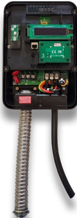
Figure 3-7 Loop EV-Flex EVSE with flex conduit attached
