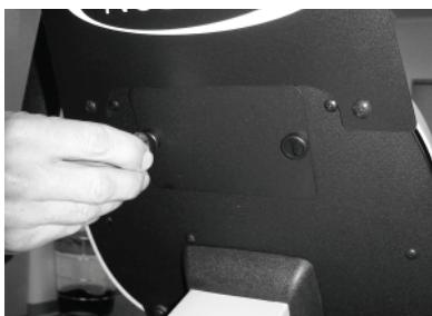
**Use coin to remove battery access panel.**
