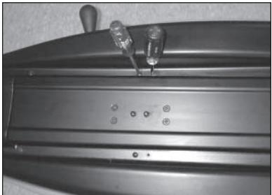
**For top cover installation, place scratch awl in third hole from front to align holes, then insert 3 screws. Repeat for opposite side.**
