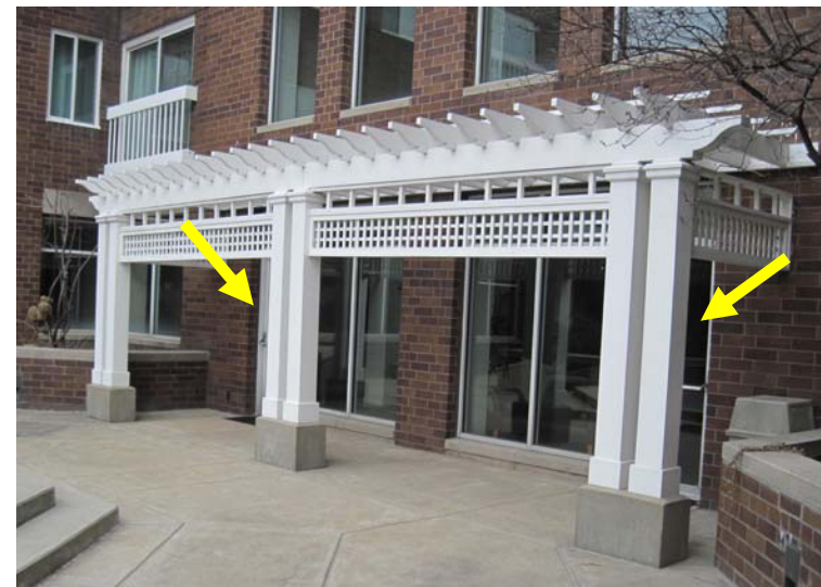
The rear courtyard entrance features two single-leaf full-lite aluminum and glass doors and low maintenance Azek PVC/polymer pergola.
